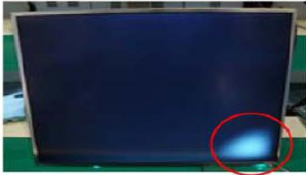
Panel Mura, Light leakage
