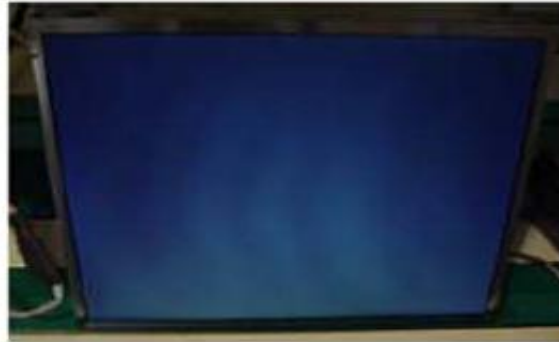
Panel Mura, Light leakage
