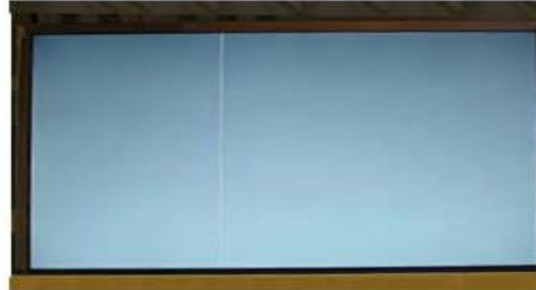
Vertical Line Source TAB IC Defect
